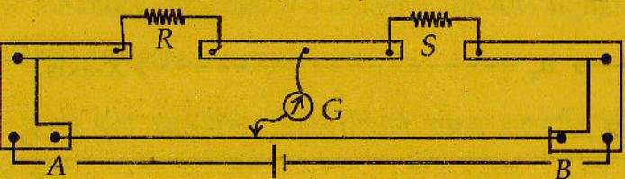
In the meter bridge shown in the above figure, the null point is found at a distance 33.7cm from A and of the wire for particular values of  $R$  and  $S$ . If a resistance of  $12\Omega$  is connected parallel with  $S$ , the null point is found to be at 48.1cm from B end. Determine the value of  $R$  and  $S$ .
